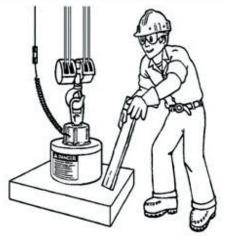
Check to be sure no one is near the load to be lifted. Inform others in the area that a lift is to begin. Lift the load 2 to 3 inches (50 to 75 mm) and then jar the load to insure that adequate holding power is available.
