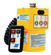
Control functions for early models of the CER magnets are labeled with: "LIFT" rather than "GRIP"
