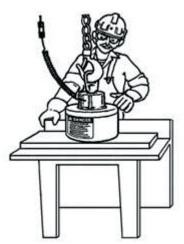
Energize the magnet by selecting the "GRIP" & "PROOF" buttons. The green indicator light will illuminate when electrical power is applied to the magnet. To obtain maximum lift, allow a few seconds for the magnet to reach full power before lifting the load.
