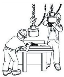
Check the condition of the magnet prior to every lift. WIPE clean the bottom of the magnet and the area on the load where the magnet will be located. File away burrs.
