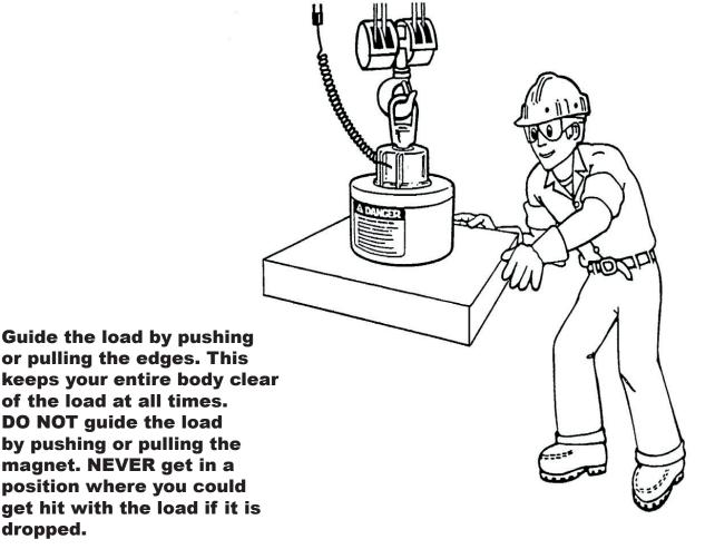
or pulling the edges. This keeps your entire body clear of the load at all times. DO NOT guide the load by pushing or pulling the magnet. NEVER get in a position where you could get hit with the load if it is dropped.
