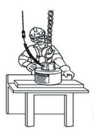
Position the magnet so the load remains level.
