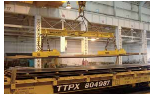
Unloading Rail Cars
