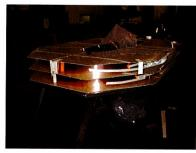
After winding, the coil is tied off with vertical straps of copper. Alcuplate is used to join the aluminum conductor to the last two turns of the copper conductor. This is one of the crucial steps that differentiates Walker Magnetics from other repair facilities. Alcuplate prevents galvanic corrosion and we are the only manufacturer to use this quality material.
