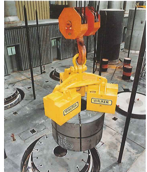
Eye-Vertical Lifting... Stack Coils in Annealing Shops
