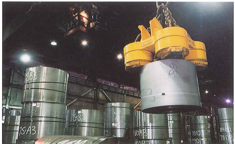
Magnetic Handling in Warehouses Allow You to Move and Stack Coils Easily
