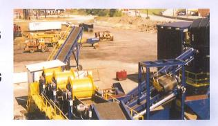
Magnetic Drums are used for separating and concentrating magnetic materials by using a stationary magnet, surrounded by a rotating shell, that imparts movement to attracted materials.
