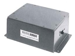
Plate Type Demagnetizers are ideal for toolroom use to demagnetize drills, cutters, ball and roller bearings, etc. The part is demagnetized by sliding it smoothly and slowly over the top of the plate, passing it clear of the demagnetizing field. The flat surface allows easy demagnetization of bulk packed nails, drills, screws, and welded parts.
