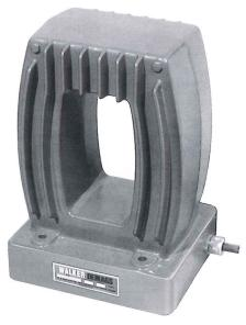
such as engine blocks, and machine casting and die blocks. The D.C. Demagnetizer uses a series of pulses of alternating polarity and decreasing amplitude to accomplish demagnetizing.
