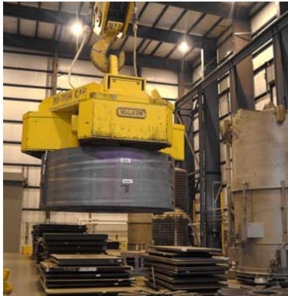
Coilmaster Magnets Move and Stack Coils Easily
