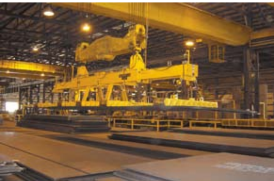
Multiple Plates with Telescoping Beam
